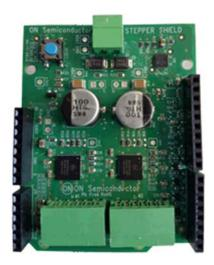
The Dual Stepper Motor Driver Shield Evaluation Board evaluates the AMIS30543, a microstepping stepper motor driver for bipolar stepper motors. It has an on chip voltage regulator, reset output and watchdog reset able to supply peripheral devices. The chip is connected through IO pins and a SPI interface with an external microcontroller that is regulated through the PCA9655E's 16 bits of General Purpose parallel Input and Output (GPIO) expansion.
