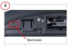
Press the bind button on the keyboard to bind it with the bridge. The mouse and keyboard work smoothly with the PC.
