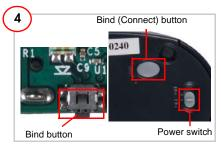
Switch on the mouse. When you press the bind button on the bridge, the red LED blinks. Press the bind button on the mouse to bind it with the bridge.
