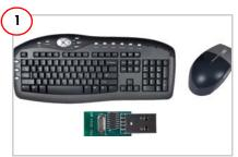
Unpack the CY4636 WirelessUSB™ LP RDK Bridge dongle, keyboard, and mouse from the package.
