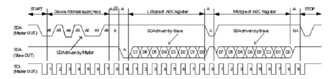
Figure 16. I<sup>2</sup>C Timing Diagram for Receive Word Format
