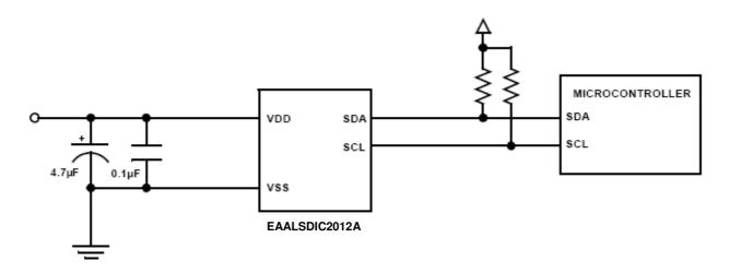
Figure 17. Application Circuit
