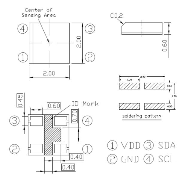
Note: Tolerances unless mentioned ±0.2mm. Unit = mm
