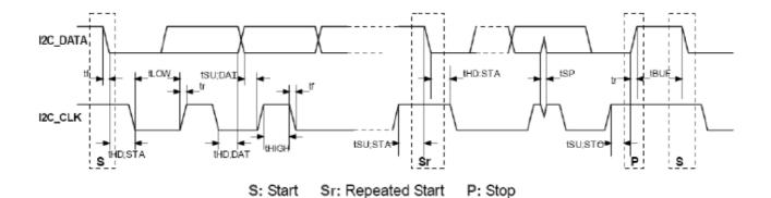
Figure 2. I<sup>2</sup>C Timing Diagram
