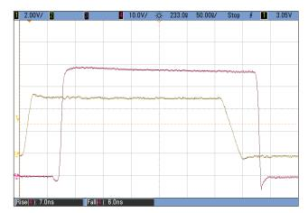
Figure 4: Typical Waveforms for  $V_{IN} = 48 \text{ V}$  to 5 V/35 A (300 kHz) Buck converter CH1: PWM input voltage ( $V_{PWM}$ ) – CH4: Switch node voltage ( $V_{SW}$ )
