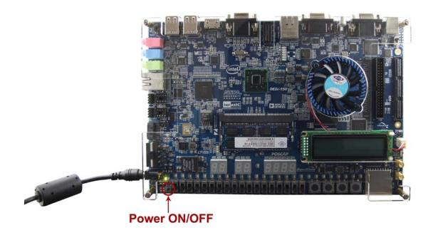
Note: Be careful not to plug the power adapter into the SATA power connector!
