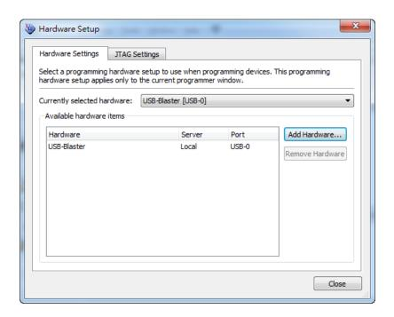
If the USB-Blaster does not appear under hardware options list, please confirm if the USB-Blaster driver has been correctly installed, and the USB cable has been properly connected between the DE2i-150 board and host computer.
