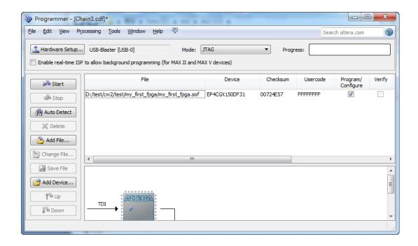
After the download has been complete, you should be able to observe that LEDG0 to LEDG3 flash in differing frequencies, meaning that the .sof has been programmed successfully.
