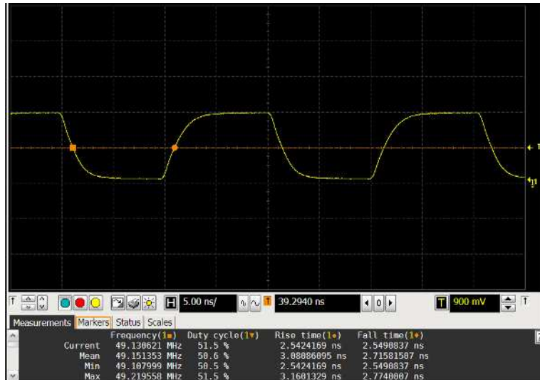
Fosc=49.152MHz、V DD =1.8V、CL=15pF、Temp=25
