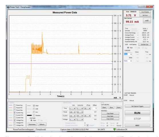
You can see the chip launch at about 1.5 seconds, then turn on the WiFi and at about 2s make the SSID connection and MQTT connection. The average current is about 100ms afterwards, and a packet spikes up to ~130mA at the 7 second mark.
