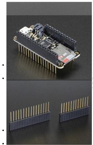
Finally, there's the "Stacking Header" option. This one is sort of the best-of-both-worlds. You get the ability to plug into a solderless breadboard *and* plug a featherwing on top. But its a little bulky
