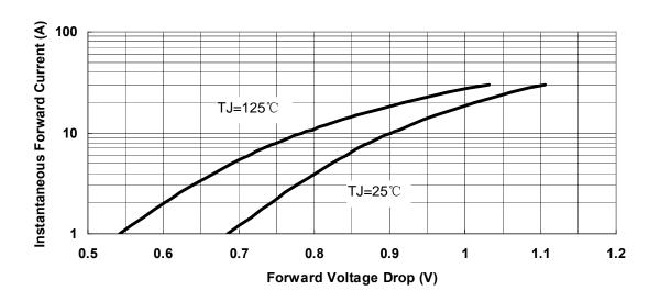
Fig.3-Typical Instantaneous Forward Voltage Characteristics
