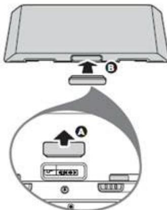
3. Align and insert the battery on the tablet PC (C).
