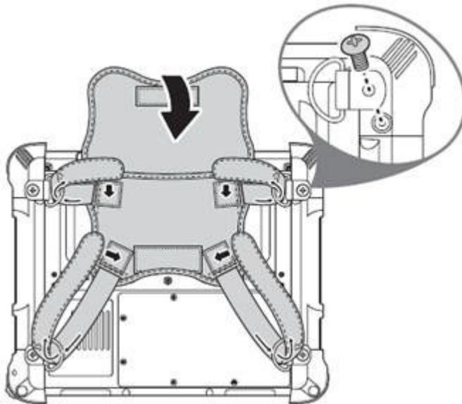
The handstrap makes it easy to carry the device on one hand.
