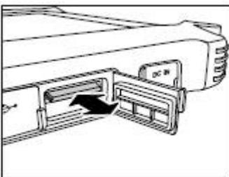
3. Remove the card and close the SD card compartment cover.
