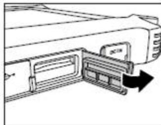
2. Insert the SD card with the metal contacts facing upwards, until it clicks into place.
