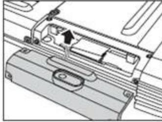
4. Attach the scanner connector to the connector inside the compartment.
