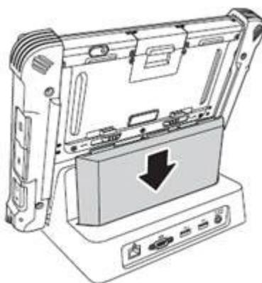
**Note!** The external battery can also be charged when installed on the tablet PC.
