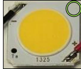
Figure 11: Soldering of SOLERIQ product
