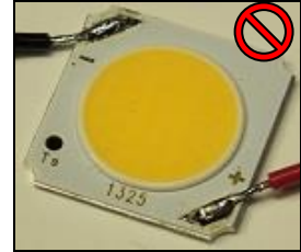
Figure 11: Soldering of SOLERIQ product
