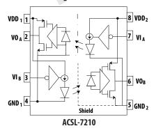
\* A 0.1  $\mu F$  bypass capacitor must be connected between pins  $V_{DD1}$  and  $GND_1$ , and  $V_{DD2}$  and  $GND_2$
