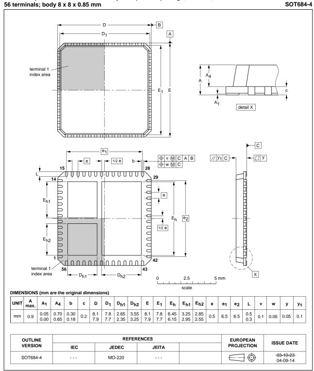
HVQFN56: plastic thermal enhanced very thin quad flat package; no leads; 56 terminals; body 8 x 8 x 0.85 mm
