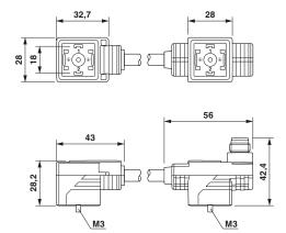
Double valve connector, 2x type A
