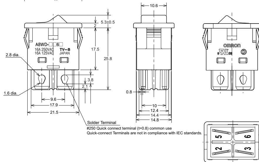
**Note:** Unless otherwise specified, a tolerance of  $\pm 0.3$  mm applies to all dimensions.
