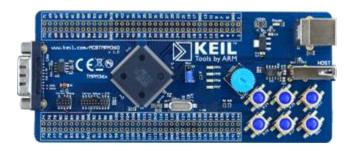
The Keil MCBTMPM360 Evaluation Boards enable you to create and test working programs based on the Toshiba TMPM360 family of ARM Cortex™-M3 processor-based devices.
