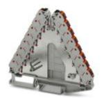
Potential distributors, Nom. voltage: 250 V, Nominal current: 17.5 A, Cross section: 0.14 mm² - 2.5 mm², AWG: 14 - 26, Connection type: Push-in connection, Number of positions: 2, Number of connections: 32, Width: 8.3 mm, Length: 100 mm, Color: gray, Color of connection elements: red, Assembly: NS 35/7,5, NS 35/15
